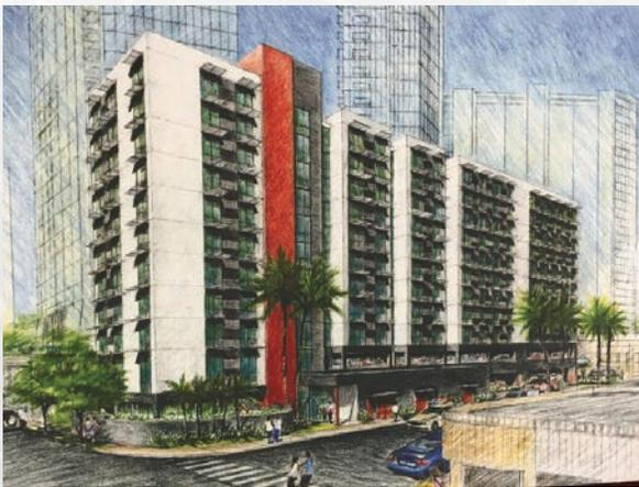
Construction is underway on this 11-story, 128-unit affordable rental project with a total height of 100 feet and approximately 153,000 GSF. Located on a constrained urban infill site the project had to incorporate parking and functional spaces under a residential tower of concrete tunnel-form construction.
