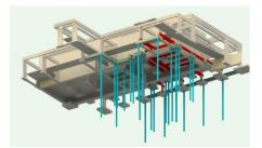
The program to provide ground settlement stabilization for the **USS Arizona Memorial Visitor Center Theaters** required a complicated shoring plan that included driving deep piles around the perimeter of the structure and threading new steel
