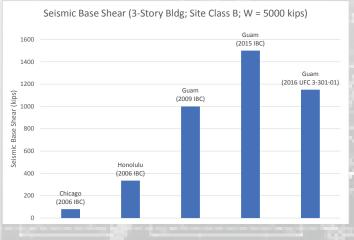
To illustrate the difference between the various seismic accelerations, the figure on the left compares the seismic base shear for a fictitious, but typical, low-rise building designed with the 2009 IBC, 2015 IBC and UFC 3-301-01. We also include the base shear for an identical building located in both Chicago and Honolulu based on the seismic accelerations in the 2006 IBC.
